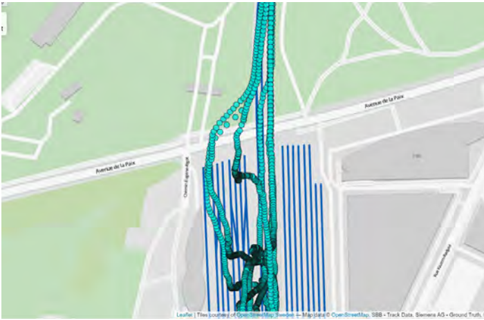
Figure 12 – Genève-Sécheron, GNSS position deviation.
