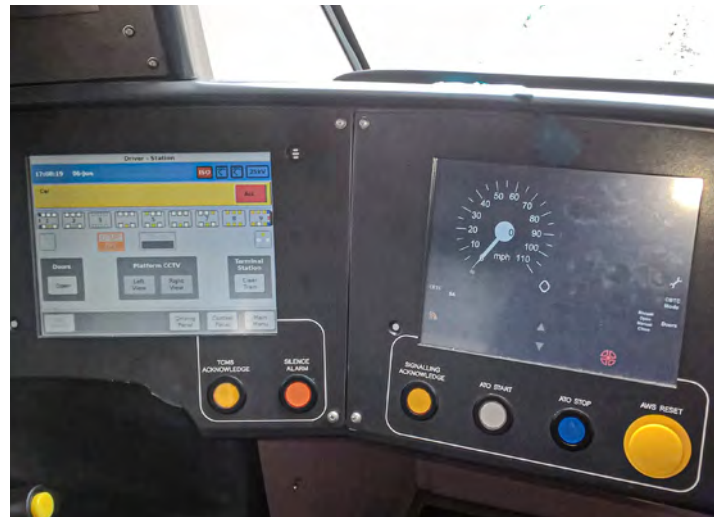
Bombardier's Elizabeth Line trains must integrate ETCS, TPWS and Trainguard CBTC. Seen here in CBTC standalone mode.
