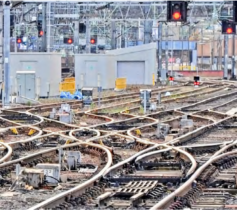
In complex areas such as Glasgow Central station, pictured left, TPWS has added a great deal of complexity to design and test in order to offer greater levels of protection than was previously available. Photo Shutterstock/DRussell78.
