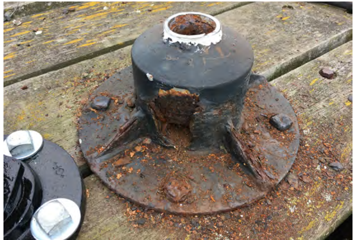
The badly corroded base for the post of key-switch T3, with the replacement post next to it.
