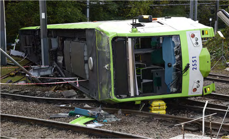
The accident on the UK's Croydon Tramlink system in 2016 resulted from overspeeding into a sharp bend.
