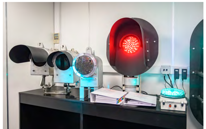
North American LED modules have been produced to convert signals from filament bulb and first-generation LED to modern LED standards.
