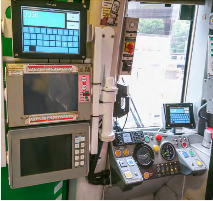
Train fitment. Left, additional operator's display in existing cab. Right, CBTC underframe interrogator transponder added.
