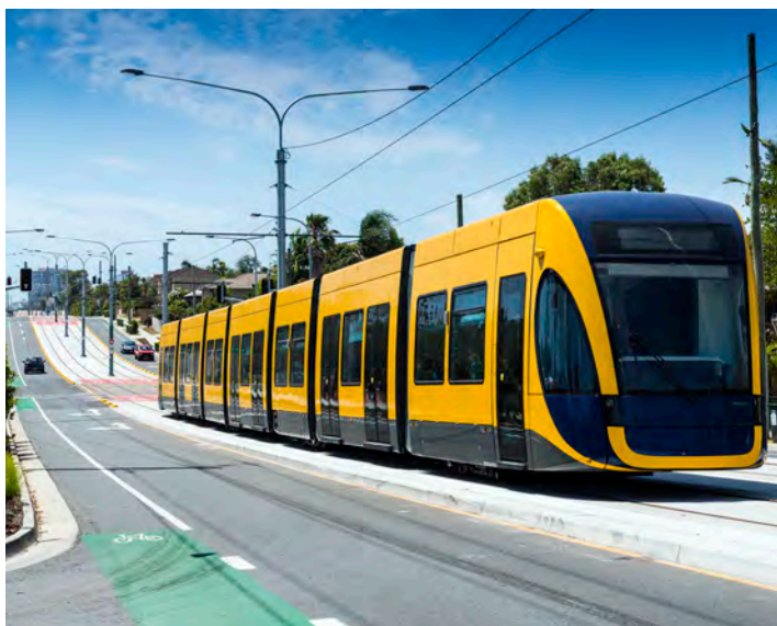
A modern low-floor light rail vehicle, in this case a Bombardier vehicle for the Gold Coast in Queensland, Australia. Photo Bombardier.
