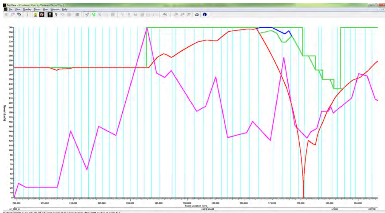
Figure 2 – Speed/distance plot showing a train checked by signals (green) compared with the free-flow speed : distance behaviour (blue).
