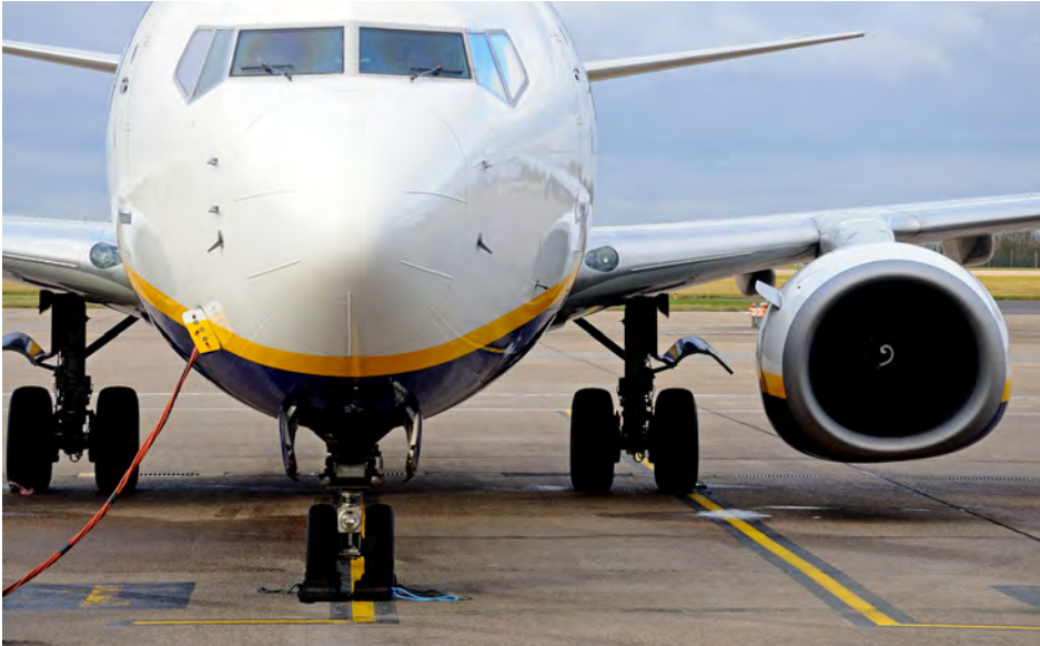
The engine nacelles of the second generation of 737s, now referred to as 737 Classic, from the 1980s onwards had a flatter bottom to allow sufficient ground clearance under the wing. Having to move the larger engines of the 737 MAX forward and higher led to design decisions that had tragic consequences. Photo Shutterstock/Caron Badkin.
