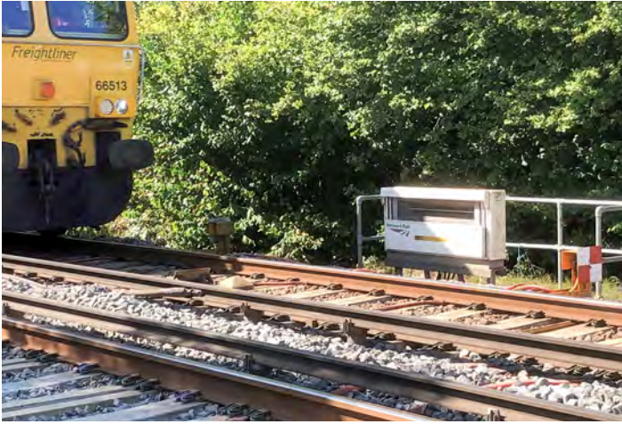
The trackside cabinet with the shutter door open and the microphone array bar just visible within.
