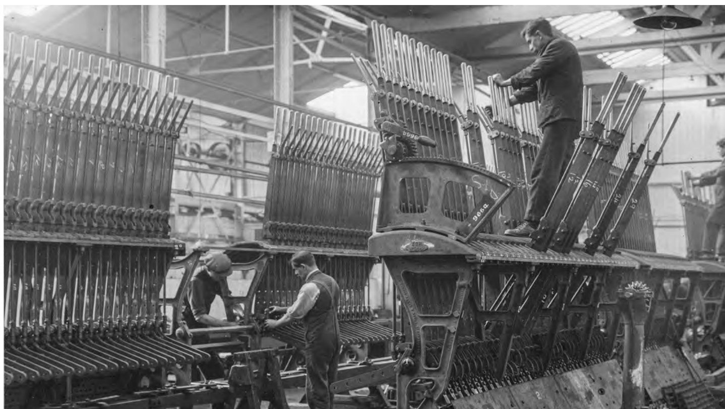
Figure 1 – The Chippenham, UK, factory of Westinghouse Brake & Saxby Signal Company in 1927. Some 60 years after the invention of the interlocking skilled teams were still assembling complex lever frames – some of which are still in use today. Photo WB&S Archive/ Chippenham Museum & Heritage Centre.
