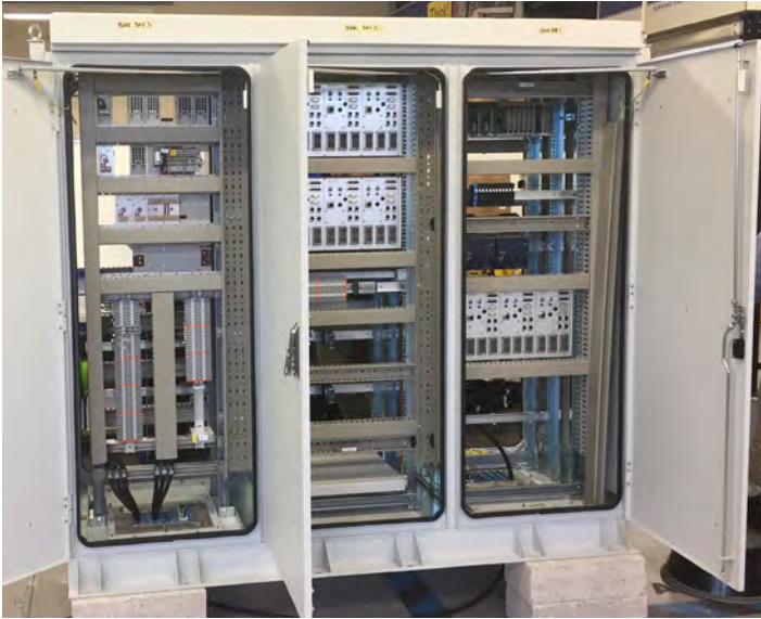
Temperature-controlled location case developed specially for the Ferriby to Gilberdyke project. Photo Arup.
