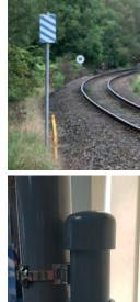
Trackside beacons can offer an effective route mile positioning system to complement GNSS positioning, especially when combined with other systems such as inertial navigation or 'wheel ticks'.
