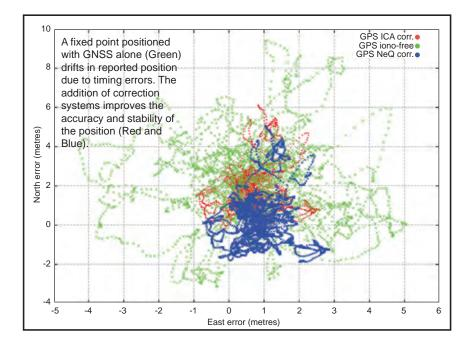
GNSS lonospheric **Distortion & GNSS** random walk GNSS signals pass through the earth's ionosphere on the way to the surface. These layers of charged particles randomly bend the path of the timing signals on their way from the satellite constellations to the ground receiver. The increased random path lengths translate to random-walk positional navigation errors for the mobile unit on the ground.
