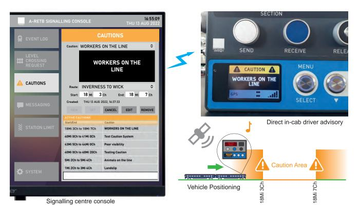
A new digital cautions reminder system allows temporary speed restrictions or other cautionary warnings to be sent directly to in-cab equipment and triggered by train position to give drivers timely caution reminders
