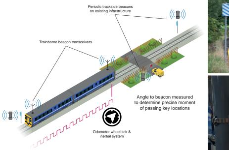
Output = track mileage + key logic (has/has not passed a key location)
