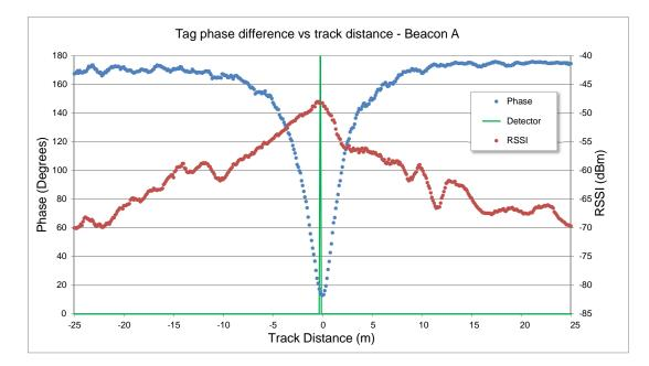
Modern IoT techniques allow trackside beacons to offer positional accuracy similar to track bed beacons for single track sections, without the installation and maintenance challenges of track bed equipment. RSSI is Received Signal Strength Indicator.
